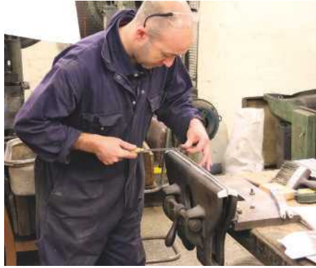
▲ The high-end saws are hand sharpened by Christian
